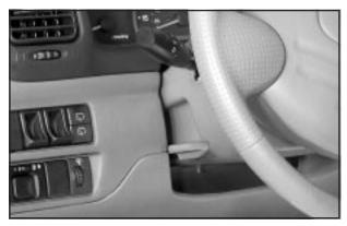
The lever that allows you to tilt the steering wheel is located on the left side of the steering wheel column.
